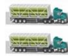
Specialised tube trailer for storage and distribution
